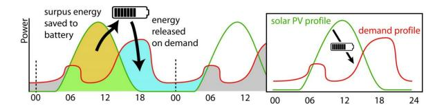
Grid solar PV has the same requirement. Battery storage (BESS) transforms a solar farm's PV generation profile into the NG demand profile.
