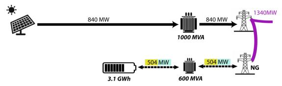
The battery's grid connection will be at least 500 MW in order to receive BWSF's surplus energy generation.<sup>3</sup>
